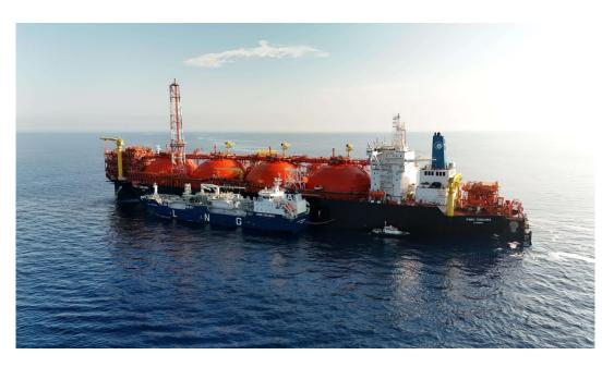
small-scale LNG service. Testina activities involved the bidirectional transfer of LNG between 7,500-cbm ING bunkering and supply vessel. Avenir Aspiration, operated by Axpo, to the TFSRU and from the unit to the small carrier. OLT said that the FSRU Toscana will be the first to provide this service in Italy. Following loading operations. small-scale LNG carriers will then be able to refuel, directly at sea,
