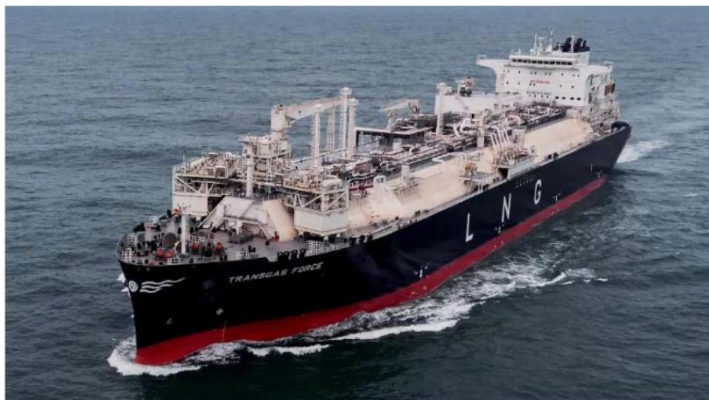
Transgas Force is among the LNG carriers due to be used as an FSRU in Europe. Source: Vesselfinder
